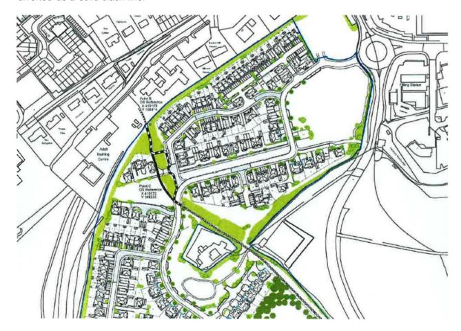
3.4 The proposed diversion will divert a 65 metre section of path and create 75 metres of path. The new route will be laid to tarmac and hoggin (a compactable groundcover that is composed of a mixture of clay, gravel, and sand or granite dust that produces a buff-coloured bound surface). The sections of footpath MARL30 that are within the development site, but do not need to be diverted, will also be improved with a surface of hoggin and a width of 2 metres will be provided.
